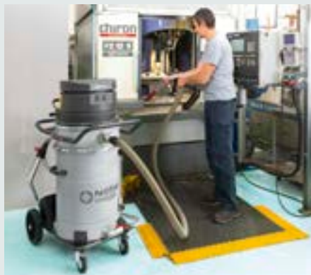
Recovery of chips and oil from a machine tool
