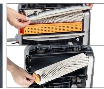
14. Remove the squeegee. Unscrew by turning the knob clockwise to remove the cylindrical brush.
