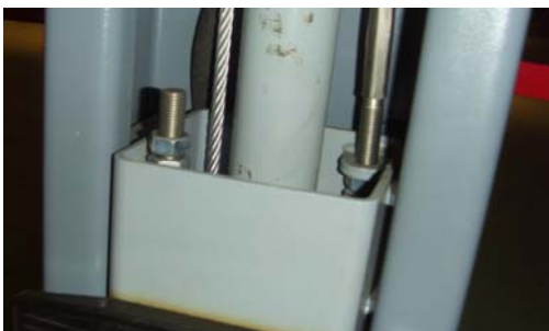
Bolt to adjust the tightness of steel cable
